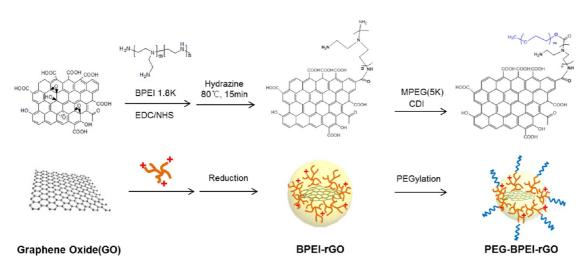
Scheme 1. Schematic illustration of the preparation of PEG-BPEI-rGO.
